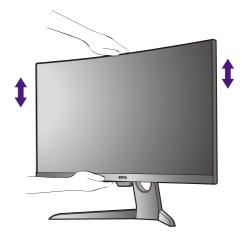
Avoid placing hands on the upper or lower part of the height-adjustable stand or at the bottom of the monitor, as ascending or descending monitor might cause personal injuries. Keep children out of reach of the monitor while performing this operation.
