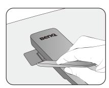
Release the screws fixing the stand to the monitor.
