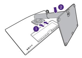
Lift the end of the monitor stand high and orient and align the stand arm with the monitor, then push them together until they click and lock into place.
