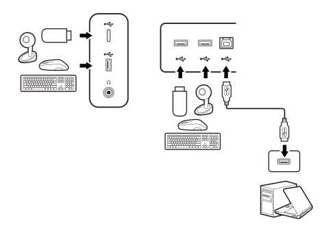
The USB-C™ port on the left or right side works as downstream port and connects with USB devices.
