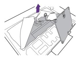
Remove the foam wrap from the monitor. Continue with Connect the PC video cable. on page 29 to complete the hardware assembly.
