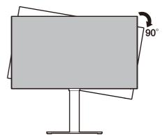
To avoid the edge of the LCD display hitting the monitor base surface while it is being rotated, do tilt and extend the monitor to the highest position before you start to rotate the display. You should also make sure there are no obstacles around the monitor and there is enough room for cables.
