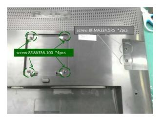
2.3 Remove Slider module from RC by Screwdriver and hand
