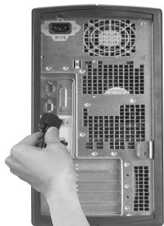
7. Connect the other end of the DVI-D cable (optional) to the signal connector of your computer.
