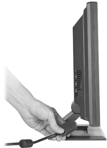
5. Open the soft cover on the back of your monitor and connect the DVI-D cable (optional) to your monitor.
