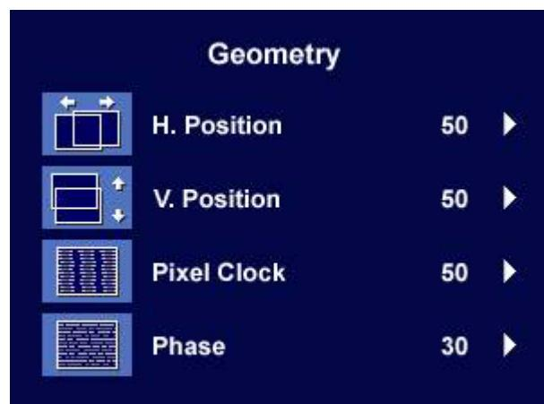
Press **◀** or **▶** key to adjust the Horizontal Position, press "Exit" to return to previous menu.
