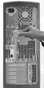
8. Connect power cord to an AC power socket.
