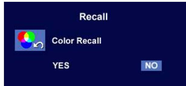
Press **◀** or **▶** key to confirm Recall All, press "Enter" key to recall position and color settings, or press "Exit" key to return to previous menu.
