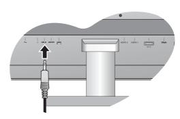
If the video source is Component, connect the corresponding audio output of your output device to the AUDIO input terminals (L/R) on the monitor using the RCA (L/R) audio cable. The plugs used for audio transmission are in white and red. Make sure that the colors of the Audio plugs and the terminals match when making the connection.
