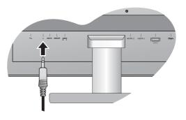
• If you prefer using external speakers, please also use another audio cable (usually supplied with the speakers) to connect the monitor (Line Out) to the input/Line In jack of the speaker.
