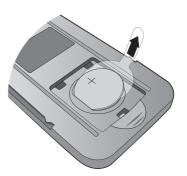
3. Replace the provided battery onto the battery holder properly. Make sure that the positive terminal (+) faces upward.
