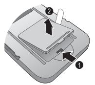
2. Remove the battery insulation sheet.
