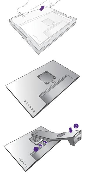
Orient and align the stand base socket with the end of the stand arm, then push them together.
