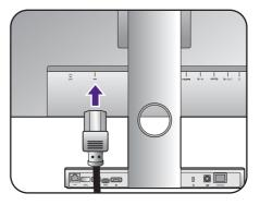
Connect the power cable to the monitor base
