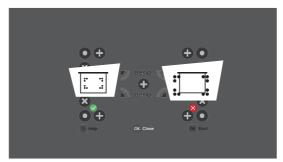
4. Press the **Auto Screen Fit** key on your remote control. The projector detects the size and ratio of the screen, and fits the focused image to the screen. Follow the on-screen instruction to complete the adjustment.
