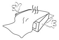
If the ventilation holes are seriously obstructed, overheating inside the projector may result in a fire.
