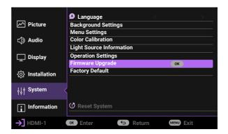
5. Select **Yes** to upgrade the firmware version. Keep the projector power on until the firmware upgrade is finished.
