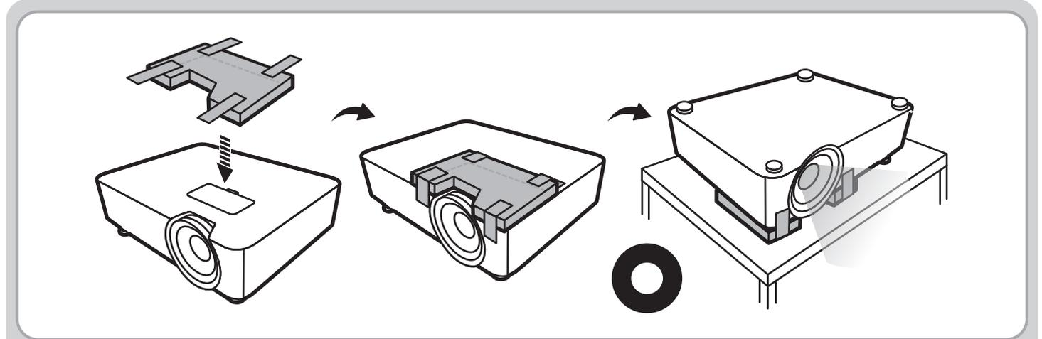
**En** In order to protect the lens, follow the illustrations above to attach the protective pad to the projector, when the projector is placed upside down on the table or the floor.
