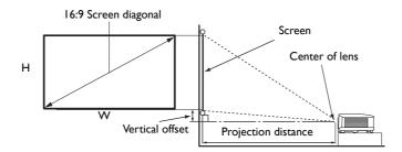
• The screen aspect ratio is 16:9 and the projected picture is in a 16:9 aspect ratio
