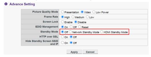
**Network Standby Mode** disables the HDMI output from the InstaShow Host after a set amount of time in which there is no connection with an InstaShow Button. When the InstaShow Host is in
