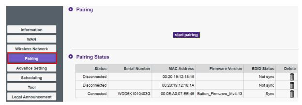
**Pairing** is used when the InstaShow Host is attached to the ceiling as it is not easy to press the **PAIRING** key of the InstaShow Host when the device is high on the ceiling. You can pair a InstaShow Button and InstaShow Host via the web management interface. See Advance Setting on page 48 for more information about EDID status.
