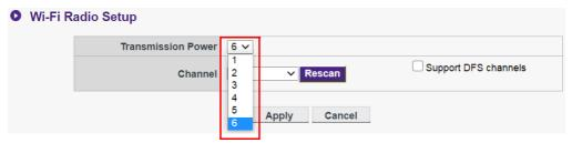
In **Channel**, you can configure the InstaShow Host to automatically select the wireless channel with the best performance during the initial setup of the InstaShow Host by selecting **Auto**, or you can select a wireless channel manually. The default **Channel** setting for the InstaShow Host is **Auto**.
