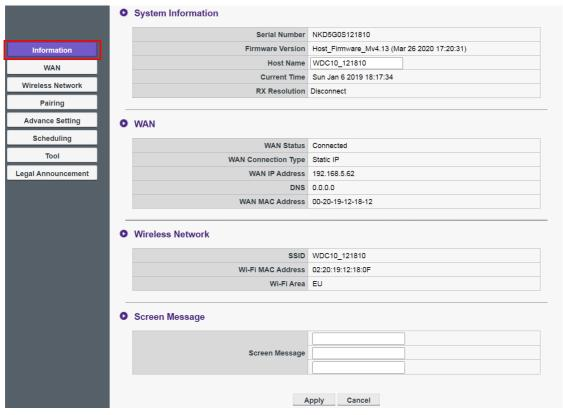
You can change the **Host Name** under **System Information**. If the Host detects resolution information being transmitted from a computer via a Button, you can find out the resolution
