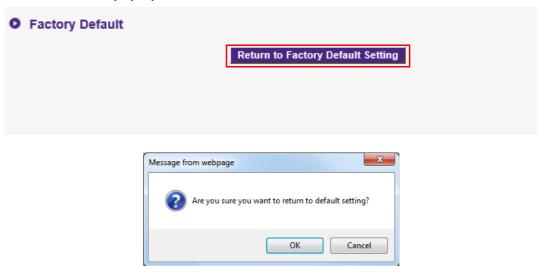
When the process is confirmed the InstaShow Host will begin restoring to **Factory Default** and the LED will quick flash red (flash red twice every second) then restart. After the InstaShow Host restarts the entire process is complete.
