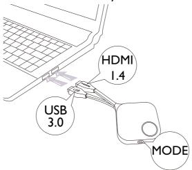
2. When the InstaShow Button is successfully connected to the laptop, the LED indicator of the InstaShow Button will blink red.
