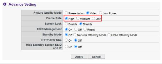
**Frame Rate** is only adjustable (its default value is set to **High**) when **Video** mode is selected. The **Frame Rate** for **Presentation** mode and **Low Power** mode are both fixed to **Low** and cannot be adjusted.
