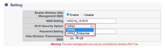
**WPA2** enables WPA2-PSK (pre-shared key) which uses an Advanced Encryption Standard (AES) encryption method.
