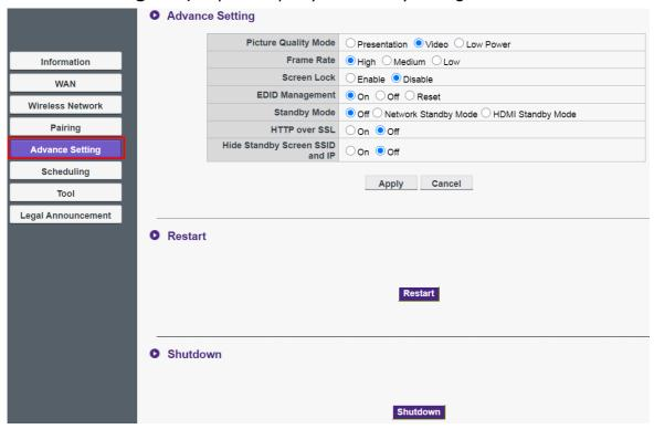
You can change mode to **Presentation** mode, **Video** mode, and **Low Power** via **Picture Quality Mode**. The default mode is **Presentation** mode. Be aware that after the firmware is upgraded to v2.01, the default mode will be changed to **Video** mode. The mode set by **Picture Quality Mode** in web management is the default mode next time when the InstaShow host restarts. That is, if the mode is **Video** mode and is switched to **Presentation** mode by the InstaShow button while playing
