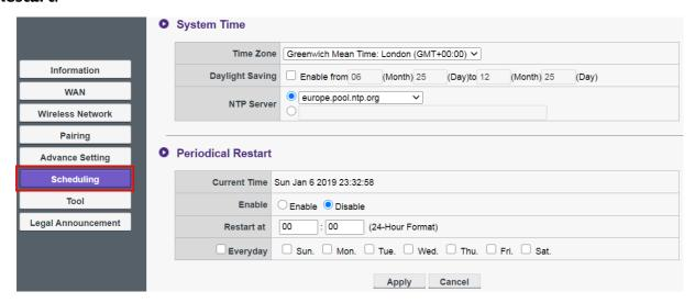
You can select your **Time Zone** and check **Enable** to set **Daylight Saving**. Select a time server from the available **NTP Server** options or input one manually to sync the system time between the Host and the browser.
