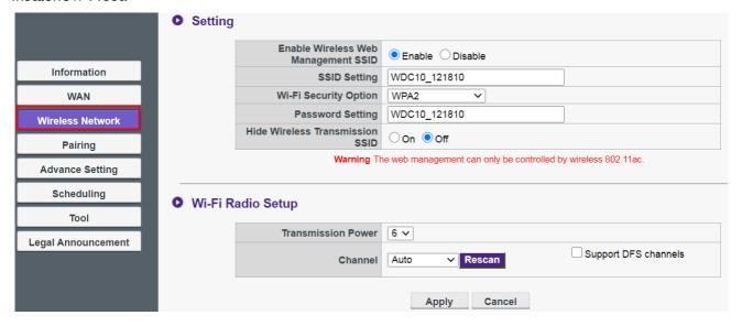
You can **Enable** or **Disable** a Wi-Fi connection to the InstaShow Host via **Enable**. The descriptions for each setting is described below:
