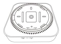
4. Attach the rubber feet to the recesses on the lid and put the InstaShow Host right next to the display.
