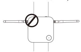
• If the InstaShow Host is attached to a metallic ceiling mount ensure that the antennas are at least 3 cm away from the metal portion of the ceiling mount:
