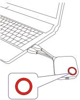
3. When the InstaShow button is ready to present, the LED indicator will turn green. Press the Present key when the LED indicator turns green.
