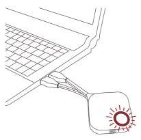
3. When the InstaShow button is ready to present, the LED indicator will turn green. Press the Present key when the LED indicator turns green.
