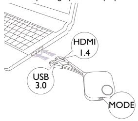
2. When the InstaShow Button is connected to the laptop, the LED indicator of the InstaShow Button will flash red. The InstaShow Button is in pairing mode, waiting to pair with your InstaShow Host.
