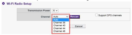
In cases when the broadcast of a presentation is unstable or choppy, due to interference to the wireless connection between the InstaShow Host and InstaShow Button from other wireless devices in the area, users can switch the **Channel** by pressing **Rescan**. By pressing **Rescan** the InstaShow Host will switch to the wireless channel with the best performance and least interference at the time.
