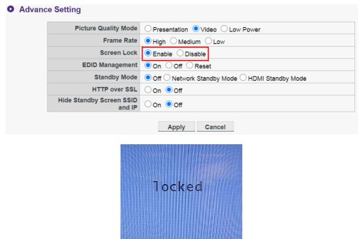
EDID (Extended Display Identification Data) is the data provided by digital displays (e.g. projectors, TVs, etc) to indicate their capabilities to its media source.
