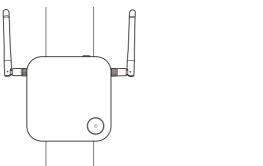
• If you encounter bad signal reception after initial use of the InstaShow Host you can manually adjust the antennas so that they tilt at a slight angle to maximize signal reception. When doing so, avoid tilting the antennas toward the ceiling mount:
