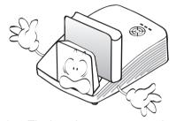
The lamp becomes extremely hot during operation. Allow the projector to cool for approximately 45 minutes prior to removing the lamp assembly for replacement.
