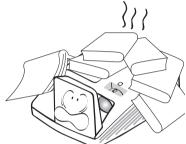
17. Do not place liquids near or on the projector. Liquids spilled into the projector may cause it to fail. If the projector does become wet, disconnect it from the power supply's wall socket and call BenQ to have the projector serviced.
