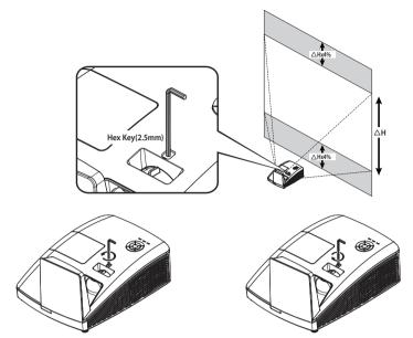
To shift up the projection image, twist the adjuster counter clockwisre.
