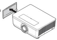
Lift the filter from the filter cover.
