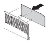
Replace the filter cover back to the projector by pushing gently in the direction shown.
