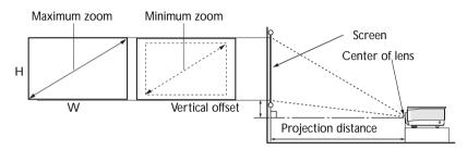
The screen aspect ratio is 16:9 and the projected picture is 16:9.
